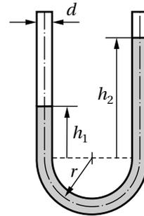
$$h_1 = 100 \text{ mm} \quad h_2 = 150 \text{ mm} \quad r = 30 \text{ mm} \quad d \ll r$$
