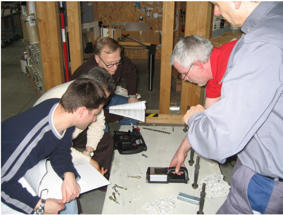
Fig. 5: A reinforcement detector helps avoiding to hit the reinforced bars [3].
