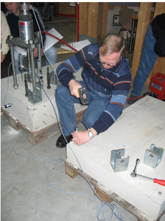
Fig. 3: The consequences of wrong assembly (here: edge distance too small) are proven in an impressive way [3].
