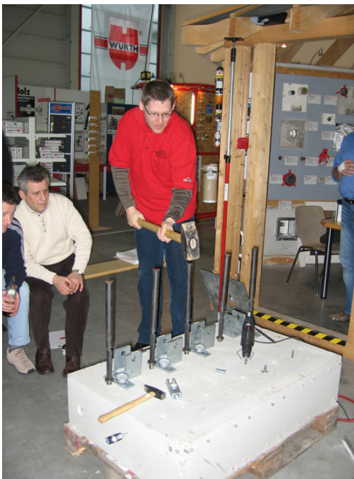
Fig 6: The tension zone (cracked concrete) is simulated [3].
