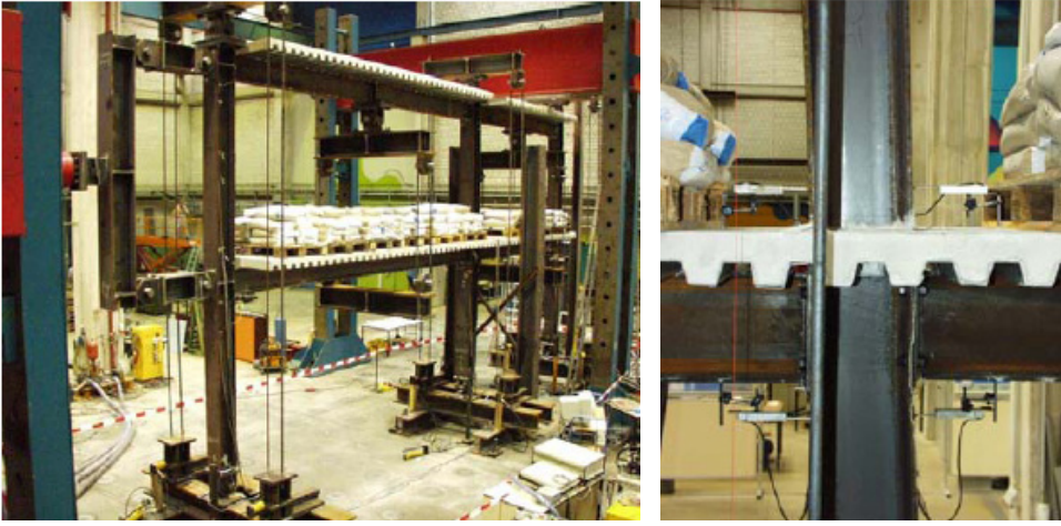
Fig. 13: Composite sway-frame test at Ruhr-Universität Bochum [29]
