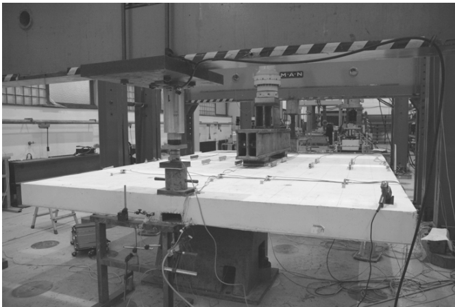
Fig. 3: Test with a slim-floor girder
